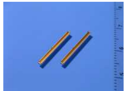
Photo 2 192-output PDP data driver IC " \mu PD16347"
